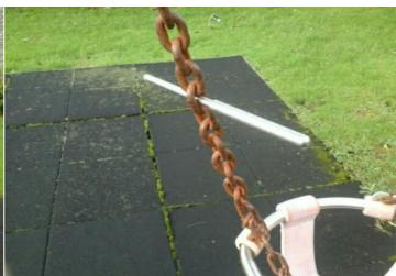
**Finding:** The chain openings are in excess of the 8.6mm as **Action:** Monitor use recommended by BS EN 1176
