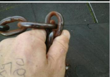
**Finding:** The chain links are worn in excess of 40% and require renewing
