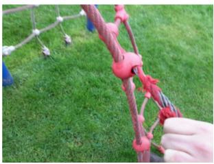
Finding: Net clamps are not secure Action: Secure
